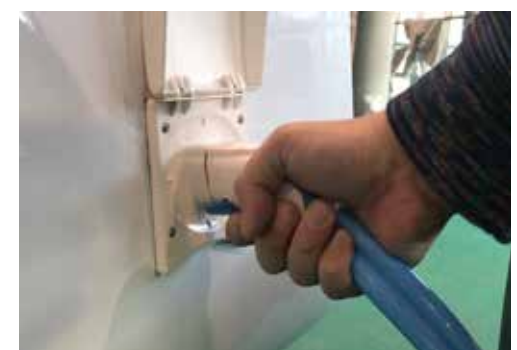
To remove, press the trigger with your index finger and pull towards you
