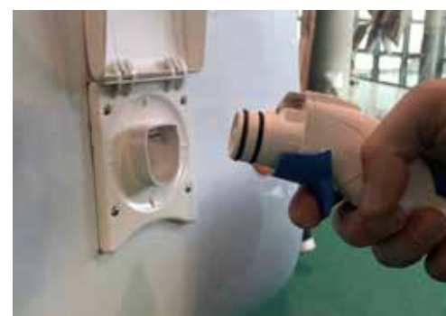
Press trigger on pump with index finger and firmly insert into socket
