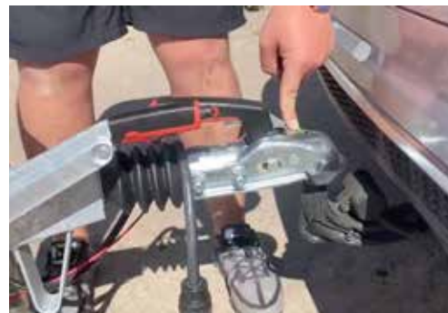
Connection is secure when handle clicks down and green indicator pops up
