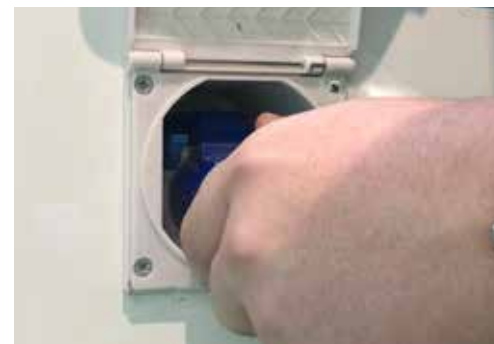
Push in firmly to ensure connection - sides must be flush
