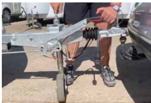
Release handbrake & move into position
