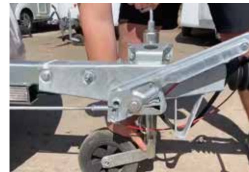
Wind jockey wheel up fully, lift & clamp into position
