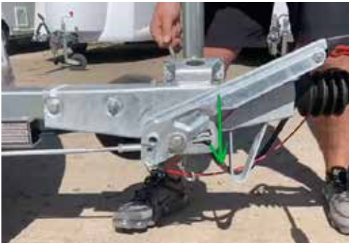
Release clamp, lower jockey wheel, re-apply clamp and wind to required height
